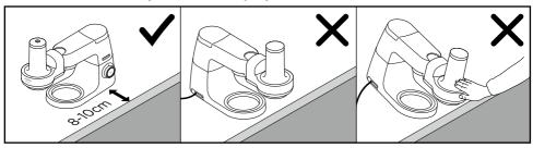
Do not move or raise the mixer head with an attachment fitted as the Stand Mixer could become unstable.
